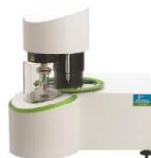
Thermogravimetric Analysis (TGA) is conducted to determine mass changes over a temperature range. This provides various testing programs for oil and water content, combustion temperature, and some reaction kinetics. At EA Labs, TGA testing programs utilize a Perkin Elmer TGA 7, and hold to standard practices for organics and metallics.
