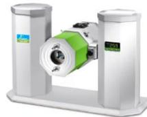
Dynamic Mechanical Analysis (DMA) is conducted on packaging material samples to determine structural stability at increased temperature. EA Labs testing holds to standard practices for organics, metallics, liquids, and powders utilizing a range of testing accessories designed for varying shapes, sizes, and physical states. EA Labs uses a PerkinElmer DMA 7e.
